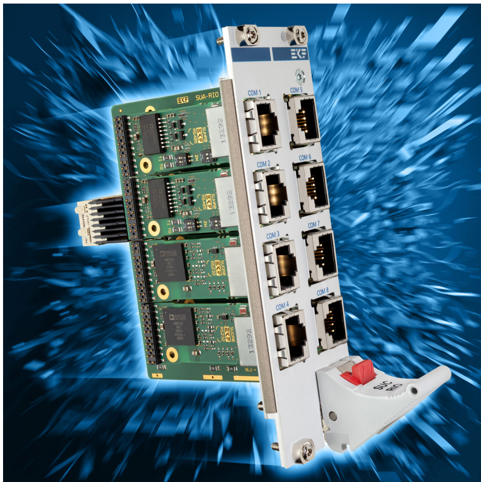
SUC-RIO 8HP (Individually Configurable RS-232/485 Ports)
